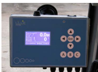
Digital logger to monitor and record every installation point
