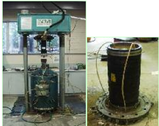
Fig. 22. Large-scale triaxial apparatus (a) Large-scale triaxial rig, (b) soil specimen
